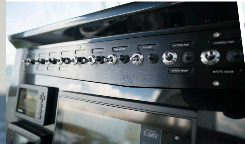
Helm console with SST switches
