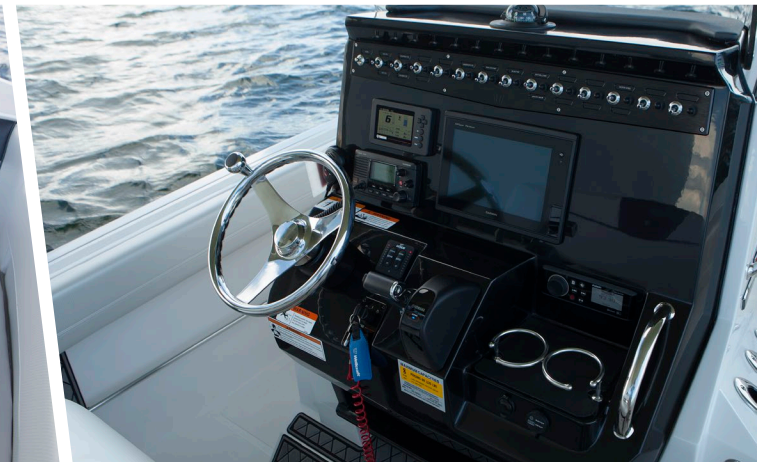
Helm center console with compass, 12 volt receptacle, SST steering wheel, and GPS plotter with depth sounder
