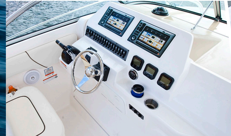
Helm console with 12 volt receptacle, compass, digital instrumentation, and SST steering wheel
