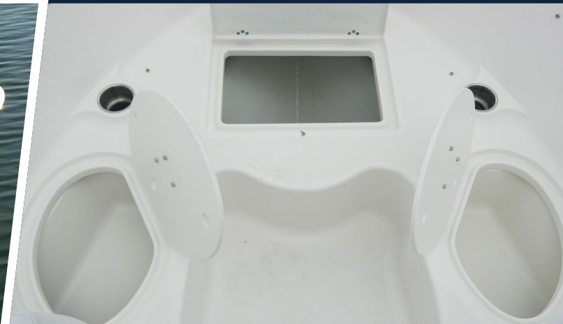
Storage/fishboxes with overboard drain
