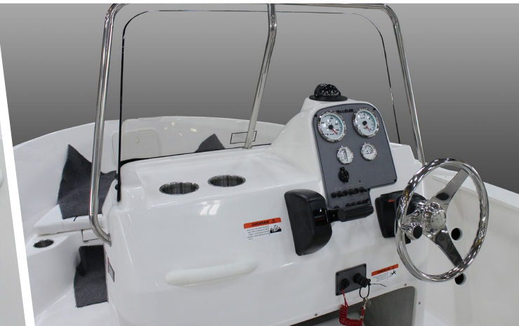
Center console with compass, 12 volt receptacle, dash instrumentation, and SST steering wheel
