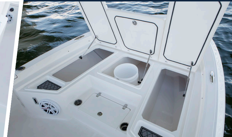
Center bow two level dry storage and 5 gallon bucket in holder
